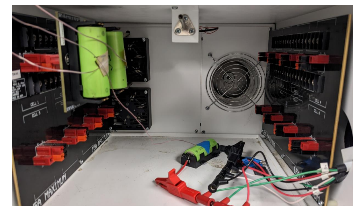
Batteries placed in a temperature control chamber to be cycled using a MACCOR Battery Tester
