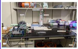
The Sample Chamber allows for the variance of bed depth, sample mass, and packing density. Nitrogen gas mass flow was controlled using an Alicat Mass Flow Controller. Pressure transducer readings on each end of the Sample Chamber were collected using a NI DAQ NI-9219 Input Module.
