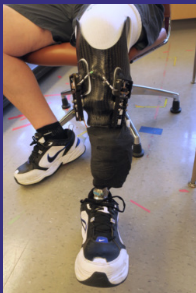
The new socket created by UW researchers automatically changes size as the user's limb changes size.
