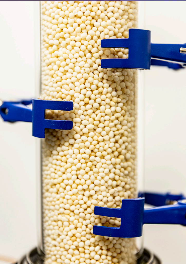
Top: Professor Emeritus Mary Lidstrom discusses the research with undergraduate Mia Grayson. Left: A close-up of a bioreactor in the lab. The cellulose beads provide a support structure for the bacteria to grow.
